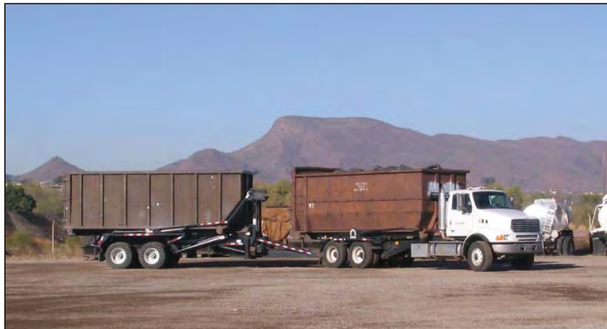
Figure 3-6: Example of Roll-off Truck with Roll-off Trailer
