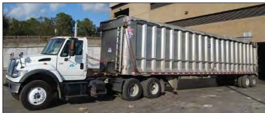
Figure 3-7: Example of Top-Load Transfer Tractor and Trailer
