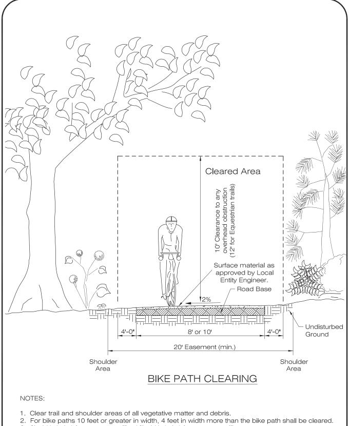
3. 8' width (min.) for one way traffic, 10' width (min.) for two way traffic.
