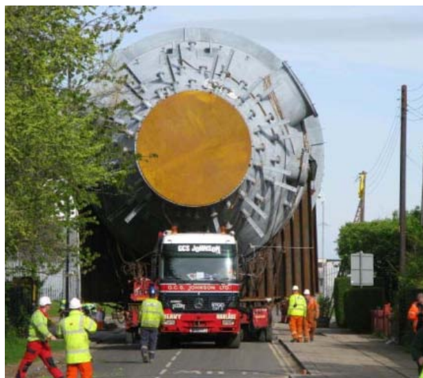
Photo #3: Alter NRG 1,000-TPD Plasma Gasification Reactor (Tees Valley, England, U.K.)
